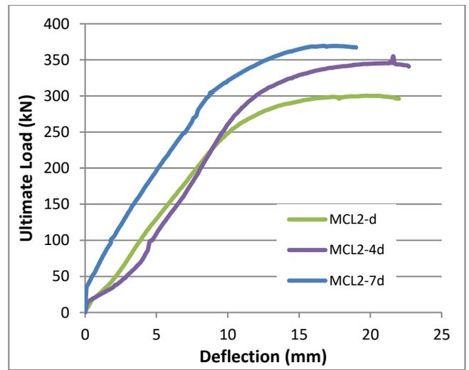
**Fig.4** Load- deflection relation for slabs with a circle-bigger column for different column distances
