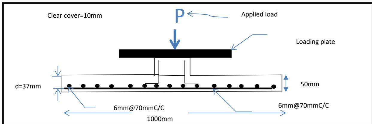
**Fig.1.** Details of specimens Cross-section and Load Arrangement to one column
