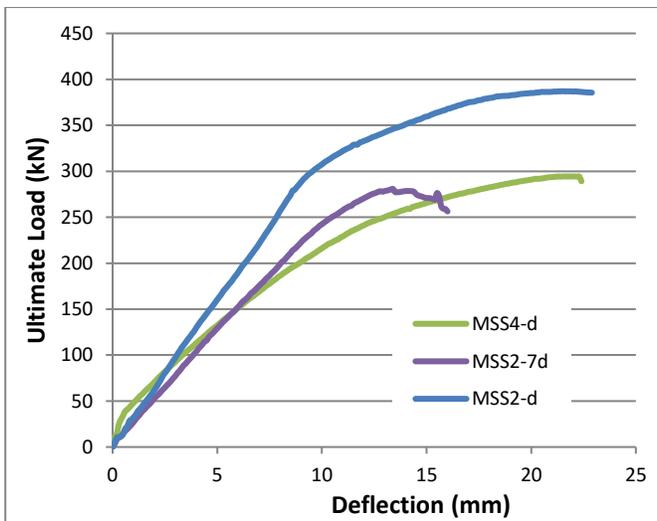
**Fig.3** Load- deflection relation for slabs with a square-smaller column for different column distances
