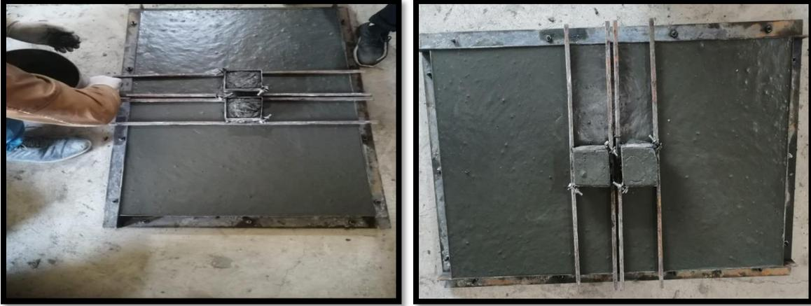
**Plate .1** Casting of slabs
