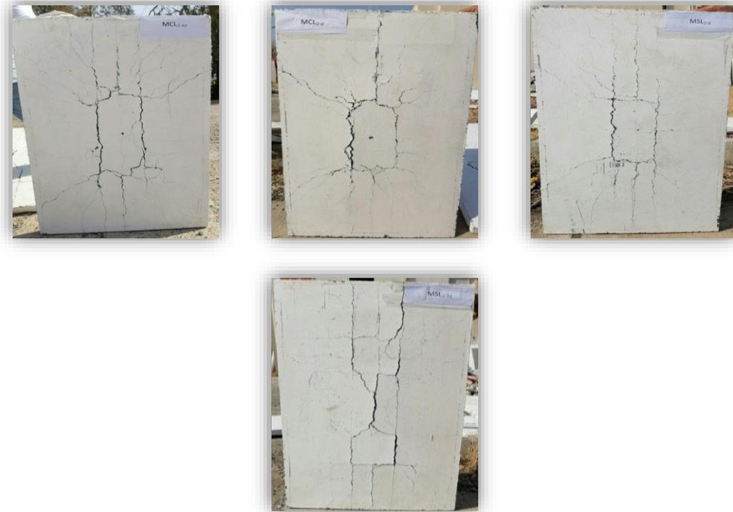
**Plate.4.** Crack Pattern for Slabs with two columns
