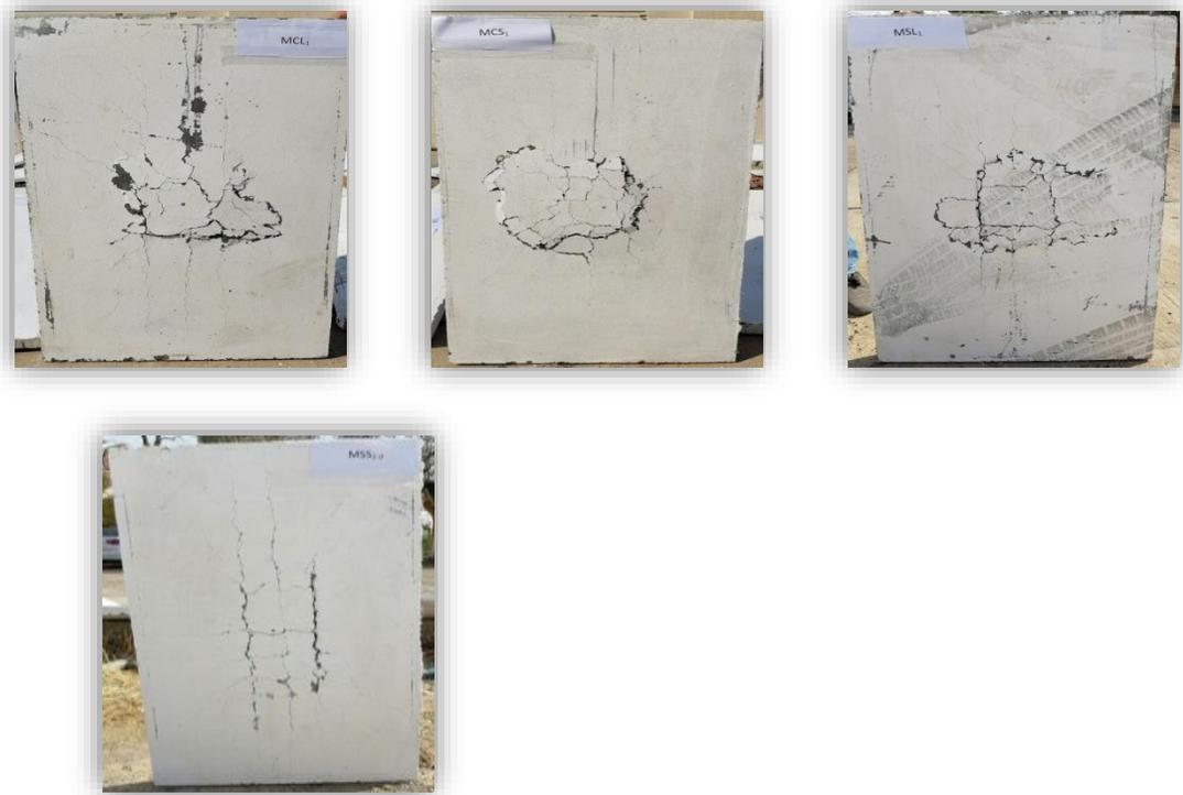
**Plate.3.** Crack Pattern for Slabs with one column.
