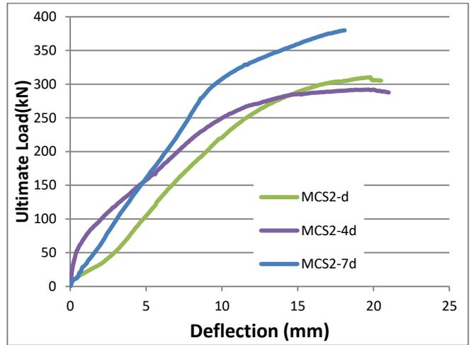
**Fig.2** Load-deflection relation for slabs with a circle-smaller column for different column distances.
