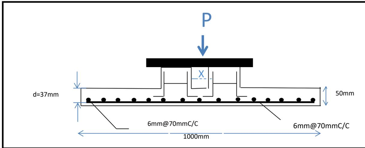
**Fig.2.** Details of specimens Cross-section and Load Arrangement to two columns.
