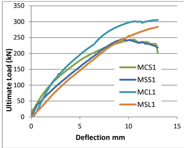
**Fig.1.** Load-deflection relationships for slabs with one column for different column section and size
