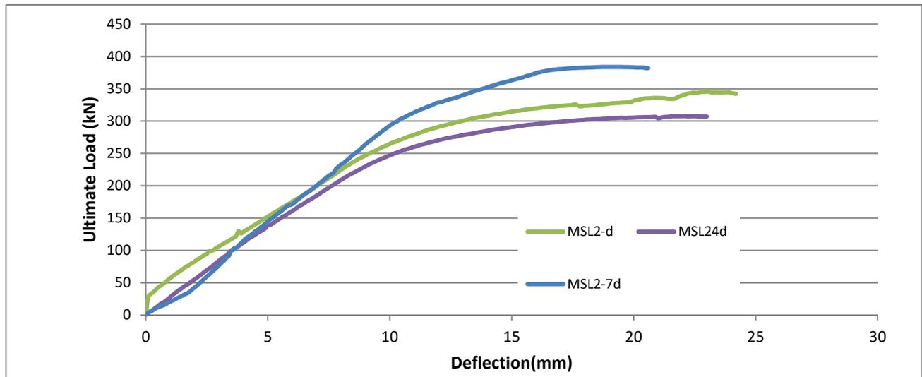
Fig.5 Load- deflection relation for slabs with square-bigger column for different column distances
