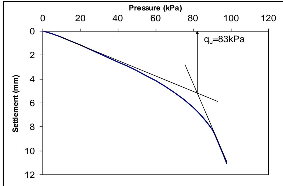
**Fig. 7 Evaluation of ultimate bearing capacity  $D_R = 72\%$ ,  $\beta = 30^\circ$ ,  $D_e/B = 2.5$**
