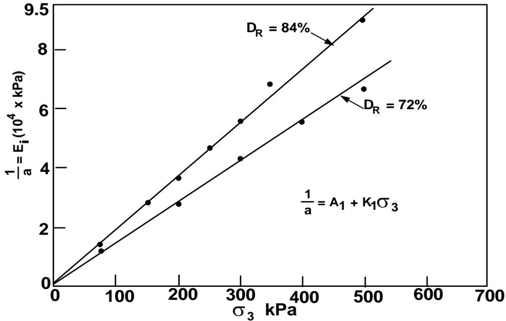
Fig. 1 Variation of  $E_i$  ( $1/a$ ) w.r.t confining pressure for Ranipure sand (After Sud, 1984)
