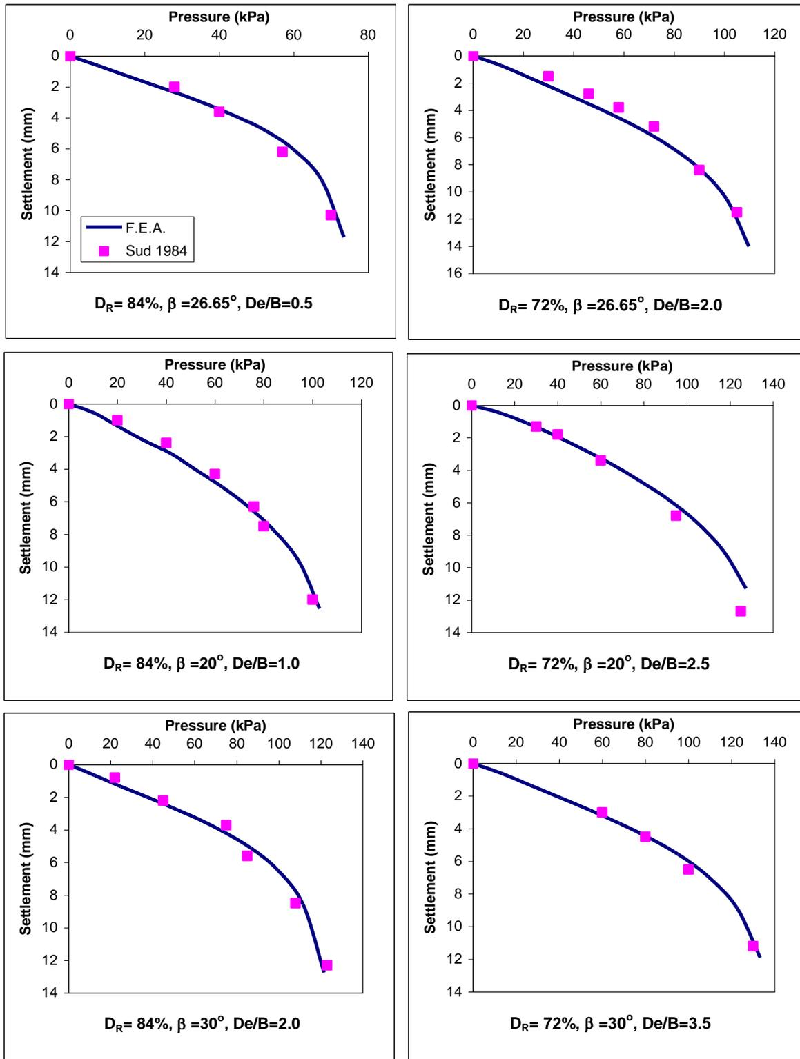
**Fig. 4 Pressure –settlement characteristics of strip footing (120 mm width)**
