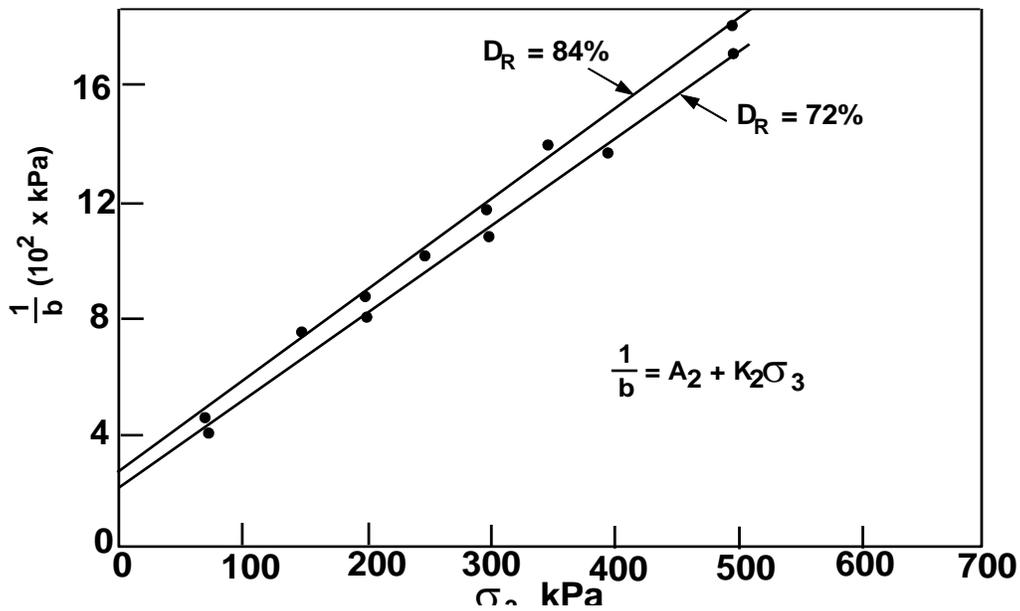
Fig. 2 Variation of Konder's ( $1/b$ ) w.r.t confining pressure for Ranipure sand (After Sud, 1984)
