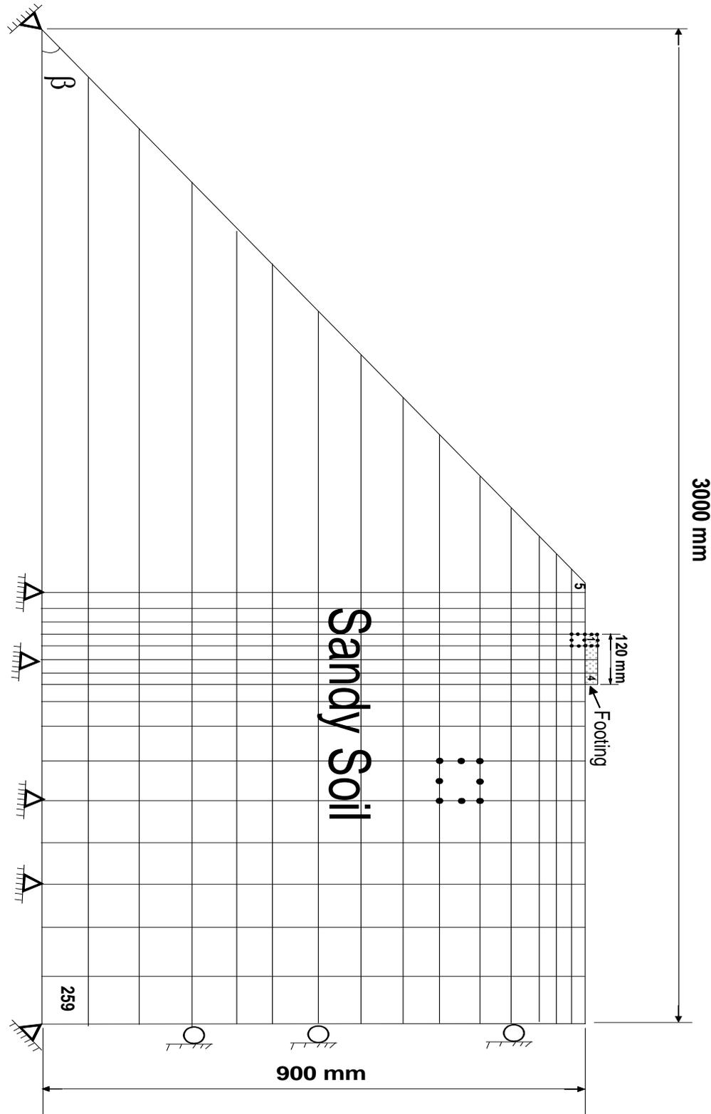
Fig. 3 F.E. Mesh representing footing –soil system (not to scale)
