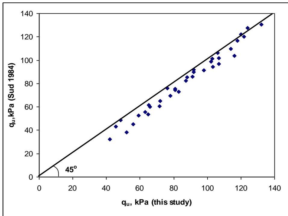
**Fig. 8 Comparison of  $q_u$  (present study) with  $q_u$  (Sud, 1984) for strip footing adjacent to slopes**
