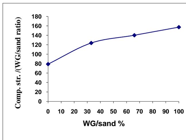
Figure (3) – the relationship between (compressive Strength / (WG/sand ratio)) and (WG/sand (%))
