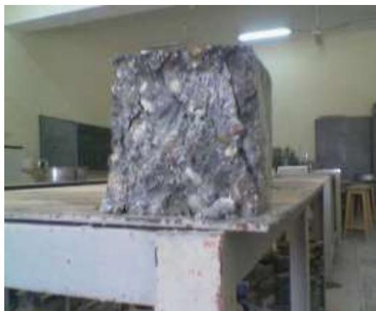
Picture (3) - shows harden cubes of (100% WG) instead of sand
