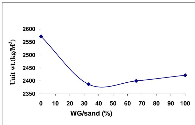
Figure (2) – the relationship between unit weights of concert and (WG/sand (%))
