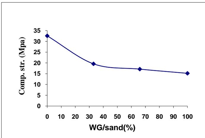
Figure (1) - the relationship between compressive strength and (WG/sand (%))
