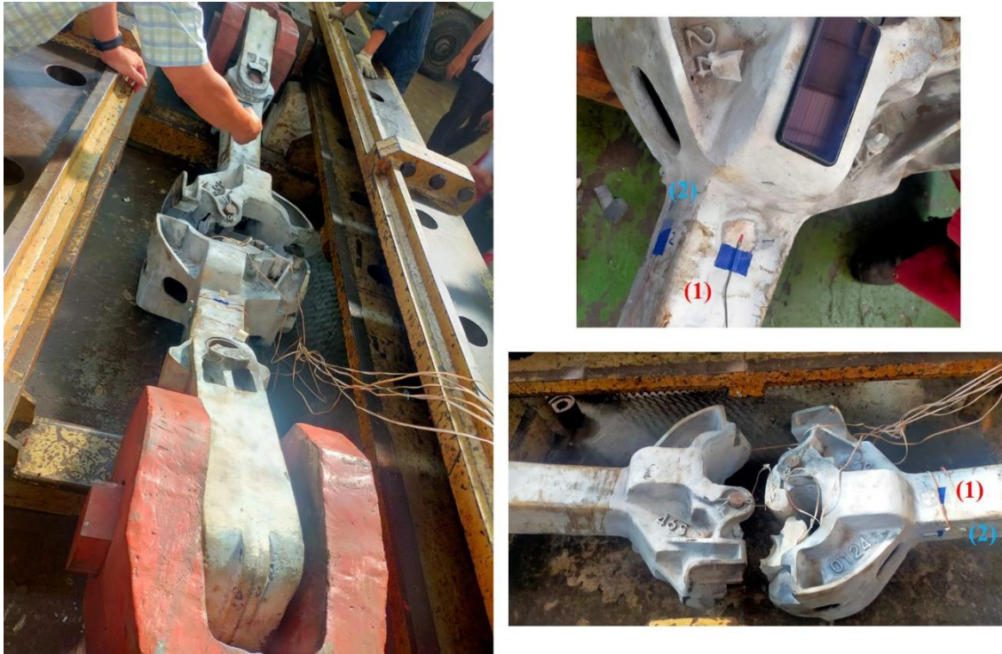
Fig. 3 Installation of Strain Gauges on Coupler Tested using RHZ 4000 Test Machine.
