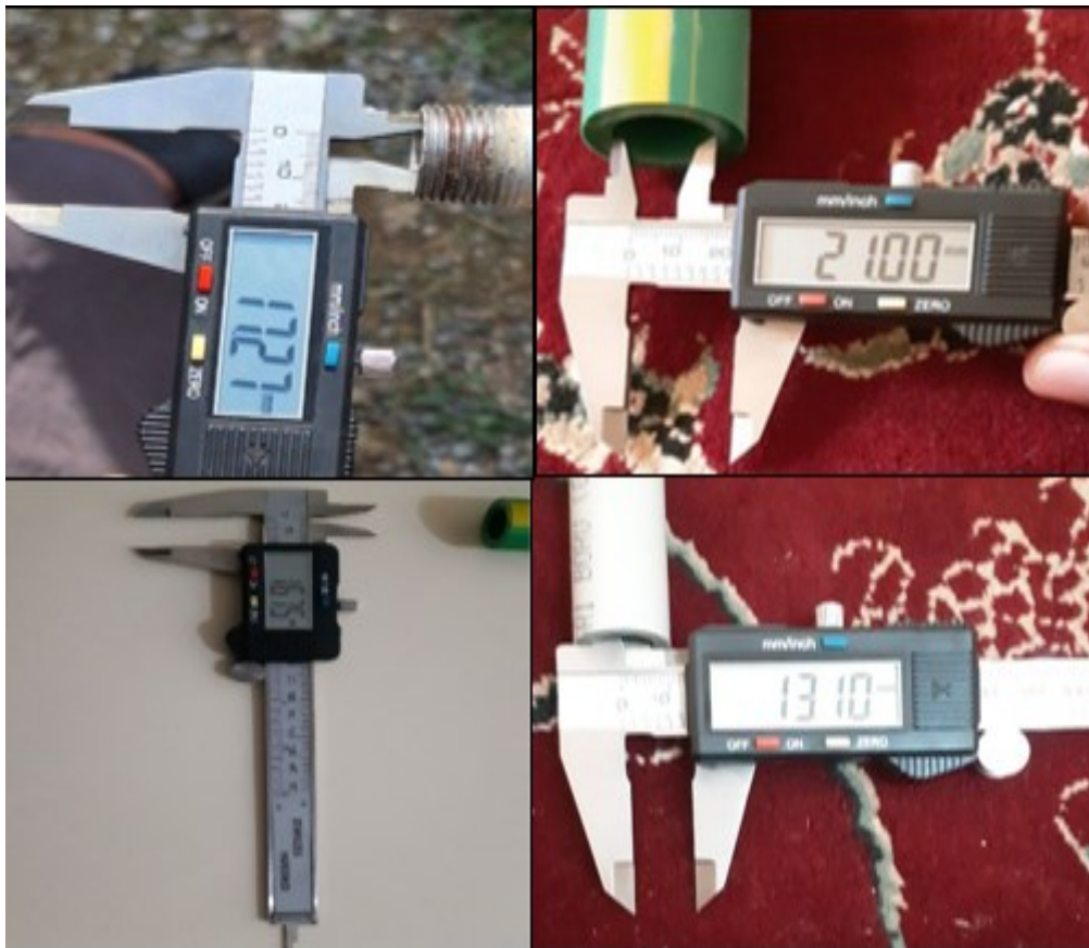
Fig. 2 Dimensions of Inner Diameter of Pipes Used in the Study.
