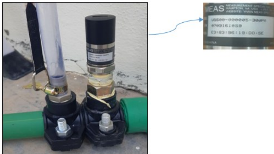
Fig. 4 Piezometer Used for Verification of Pressure Sensors
