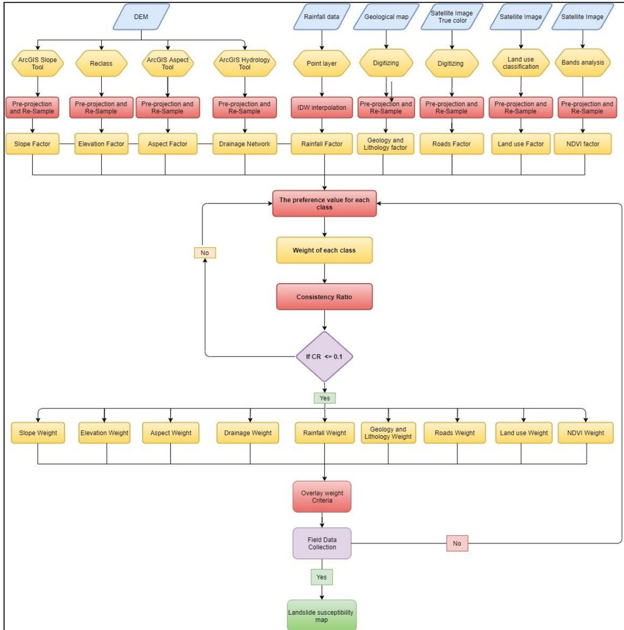
Fig.4. flowchart of landslide processes.
