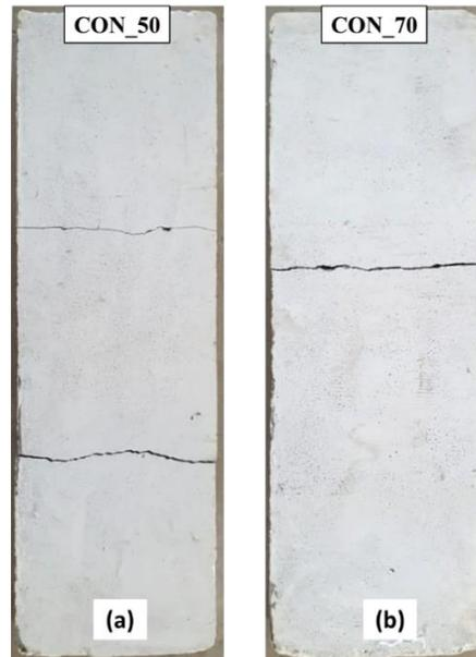
**Fig. 7.** (a) The failure mode for the control specimen with thickness 50mm, (b) The failure mode for the control specimen with thickness 70mm
