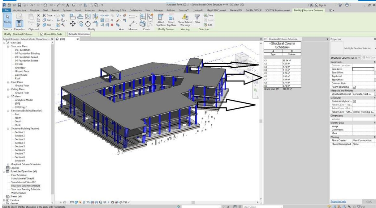
**Fig. 17** Automatic Chart and Bill of Quantities Linkage for Any Item Using BIM.
