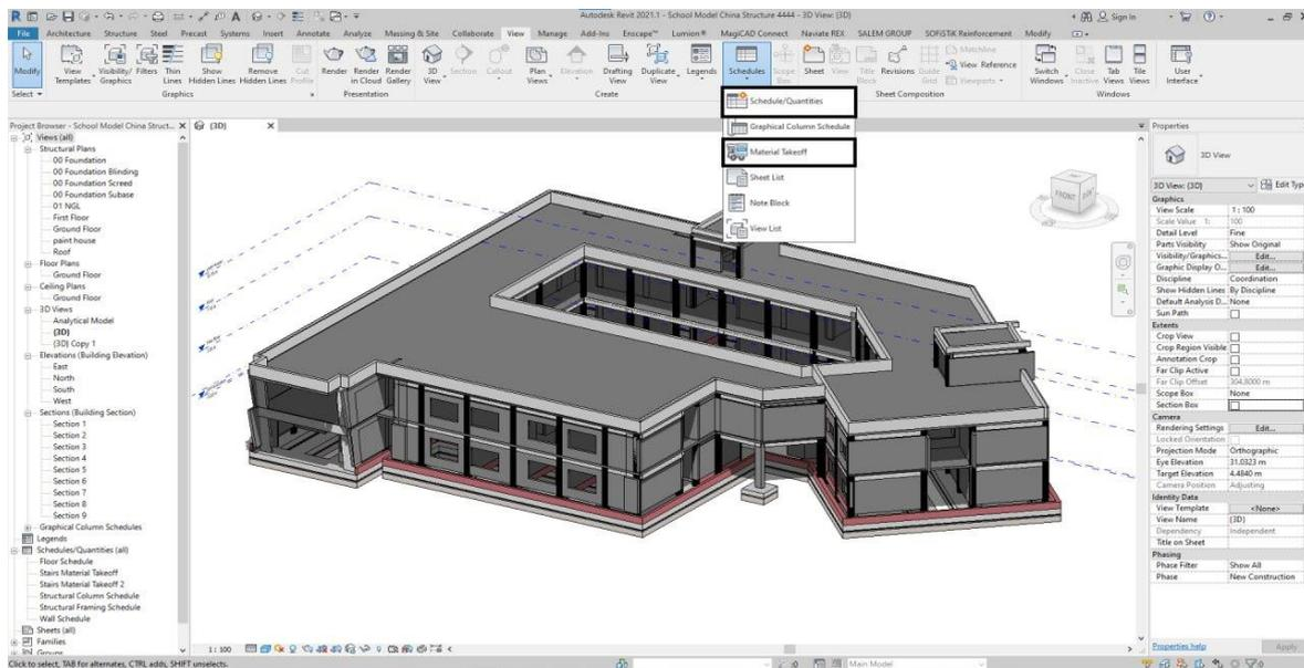
Fig. 15 BIM Tools for Calculating Quantities of Main School Building.
