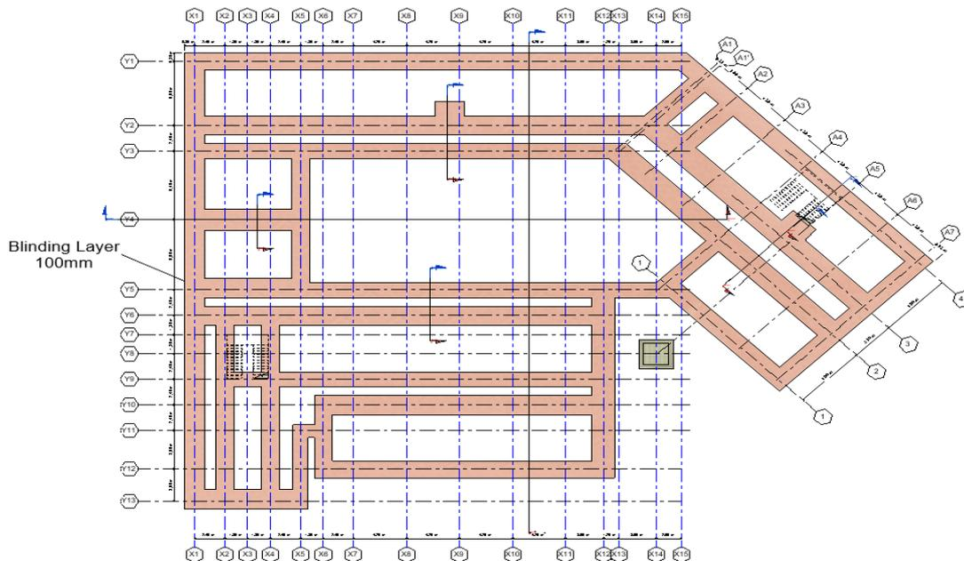
**Fig. 6** Blinding Concrete Layer for Main School Building.
