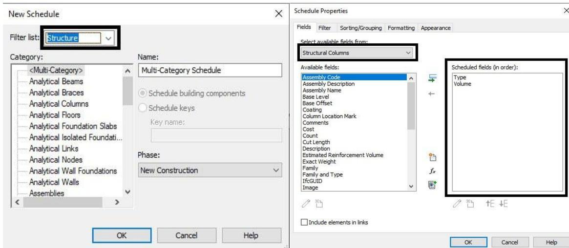
Fig. 16 The Revit Process for Obtaining Quantities.
