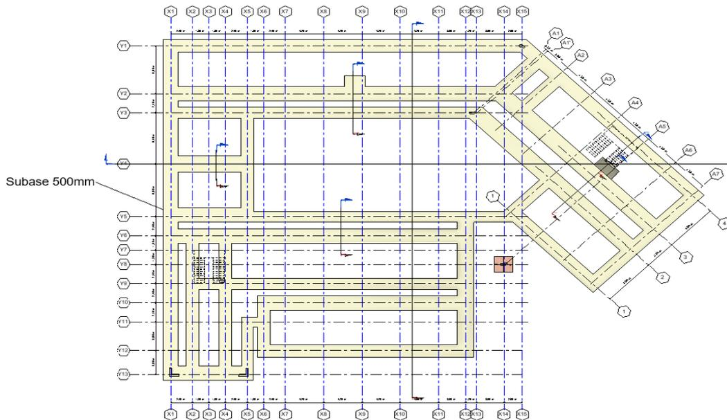
**Fig. 5** Backfilling with Sub-Base Materials for Main School Building.
