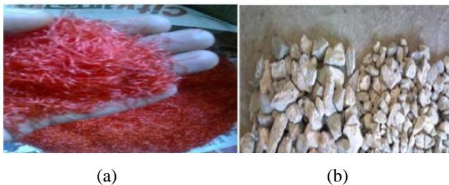
Fig. 7. (a) Polypropylene fiber (b) Recycled aggregate [30].
