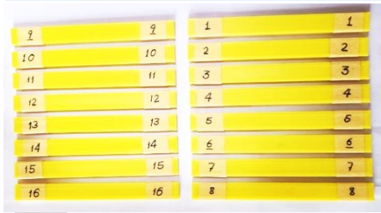
Fig. 3 Fabricated Samples for a Three-Point Flexural Strength Test.
