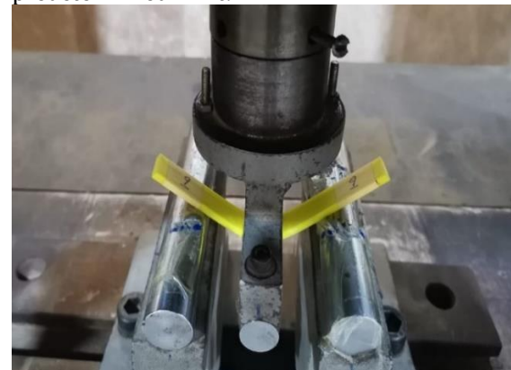
Fig. 5 Three-Point Flexural Test of a Sample.
