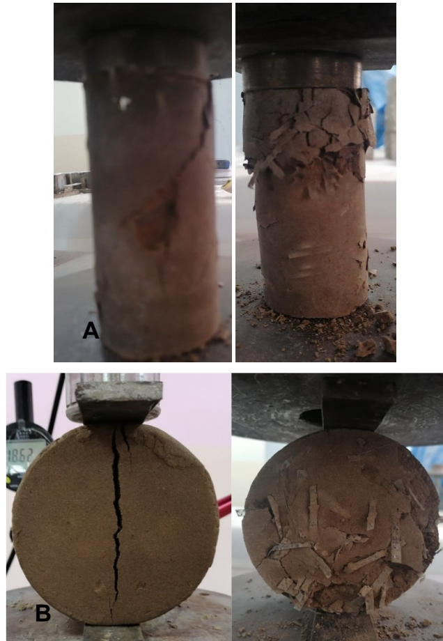
Fig. 5 Typical Failure Mode of Natural and Reinforced Soil Samples (A) UCS Samples (B) ITS Samples.
