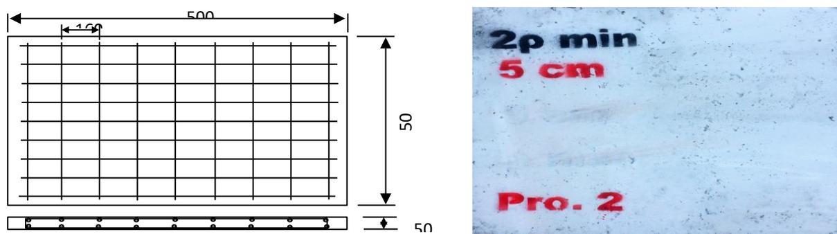
**Fig.2** Reinforcement details and casted specimen of 50 mm slab.
