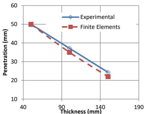
**Fig. 9.** Penetration-thickness curve for plain concrete specimens under 700 m/s velocity. For this reason, linear relationship can be drawn between penetration
