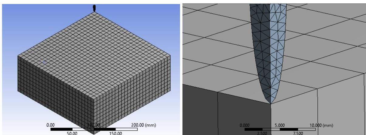
Fig.7 Slab and projectile meshing
