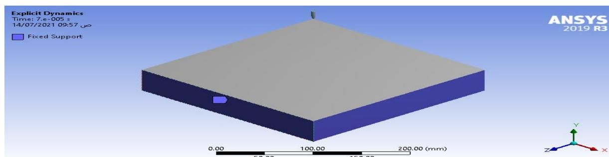
Fig. 8 Fixed supports and projectile impact loading.
