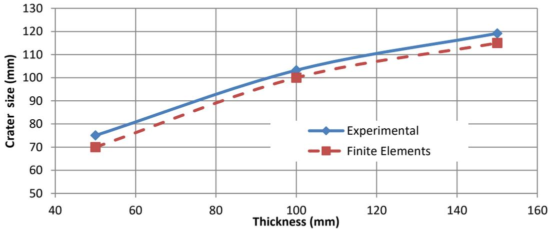
Fig. 14. Crater size-thickness curve for plain concrete specimens under 700 m/s velocity projectile
