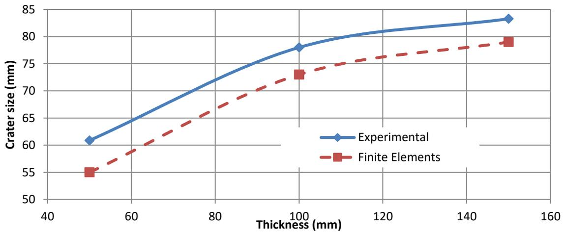
Fig. 17 Crater size-thickness curve for reinforced concrete specimens under 700 m/s velocity projectile
