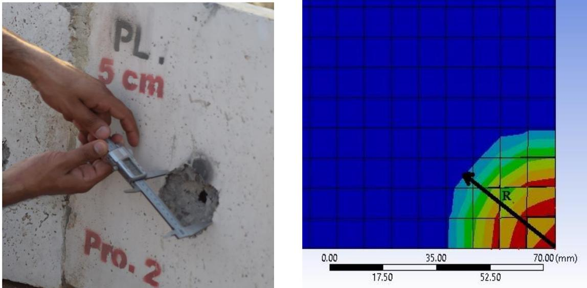
Fig. 15. Experimental and FE crater illustration
