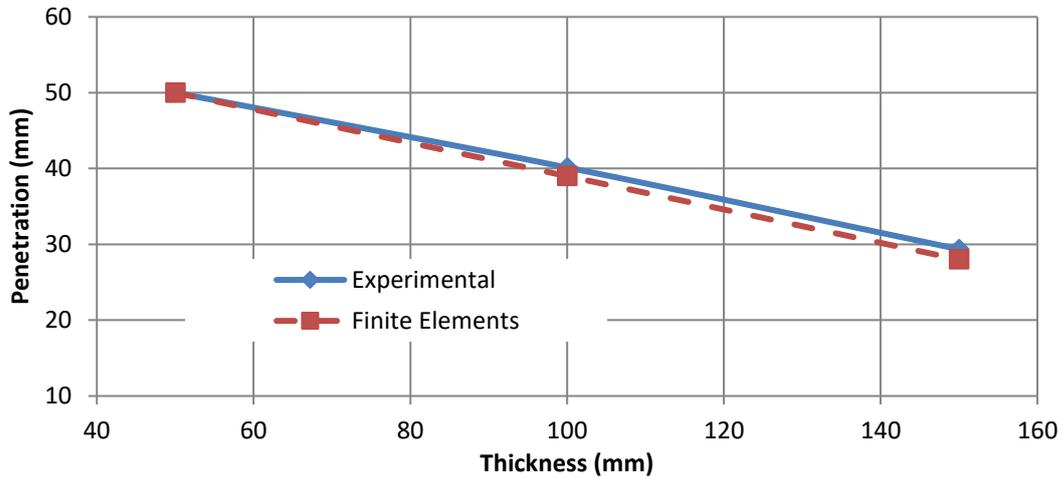
**Fig. 10.** Penetration-thickness curve for plain concrete specimens under 900 m/s velocity projectile
