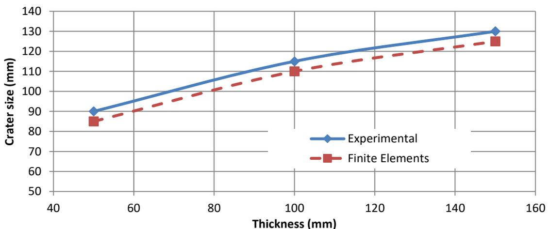
Fig. 16 Crater size-thickness curve for plain concrete specimens under 900 m/s velocity projectile
