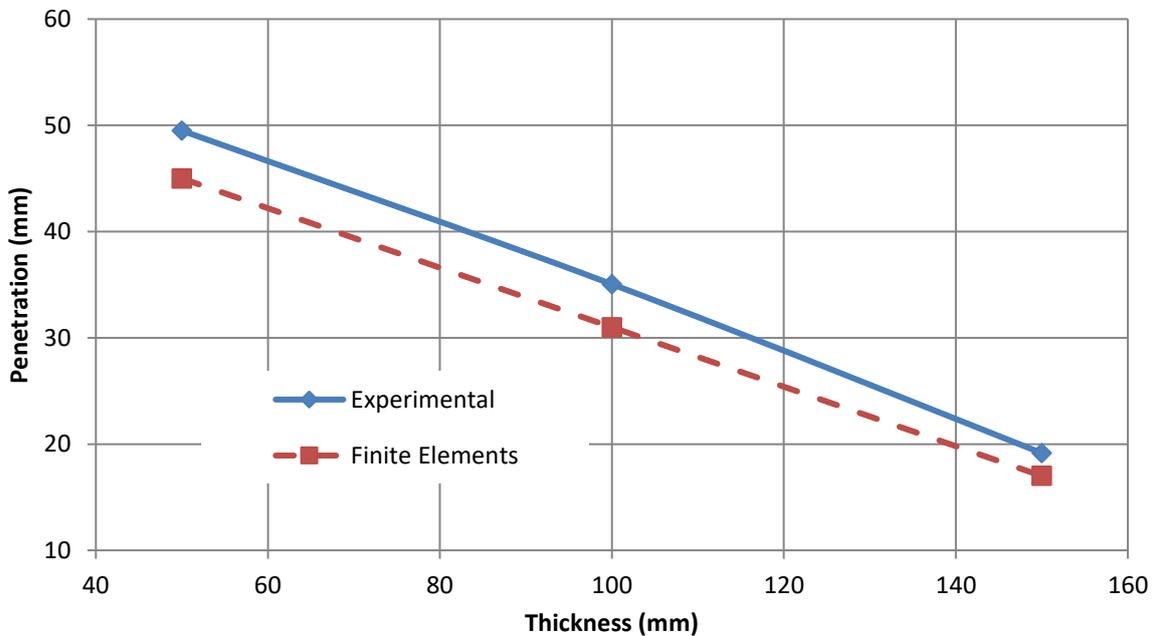
**Fig. 11.** Penetration-thickness curve for reinforced concrete specimens under 700 m/s velocity projectile
