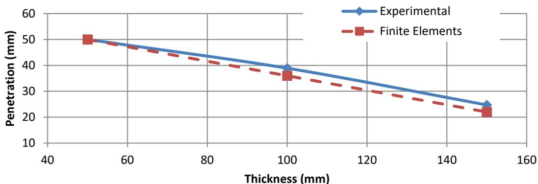
**Fig. 13.** Penetration-thickness curve for reinforced concrete specimens under 900 m/s velocity projectile
