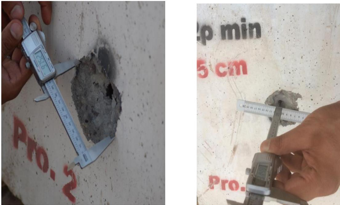
Fig. 3 Recording the crater size and penetration depth.
