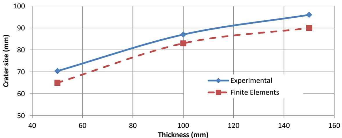
Fig. 18 Crater size-thickness curve for reinforced concrete specimens under 900 m/s velocity projectile
