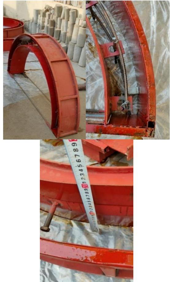
**Fig. 9** Arch Beams Steel Molds and Reinforcement.
