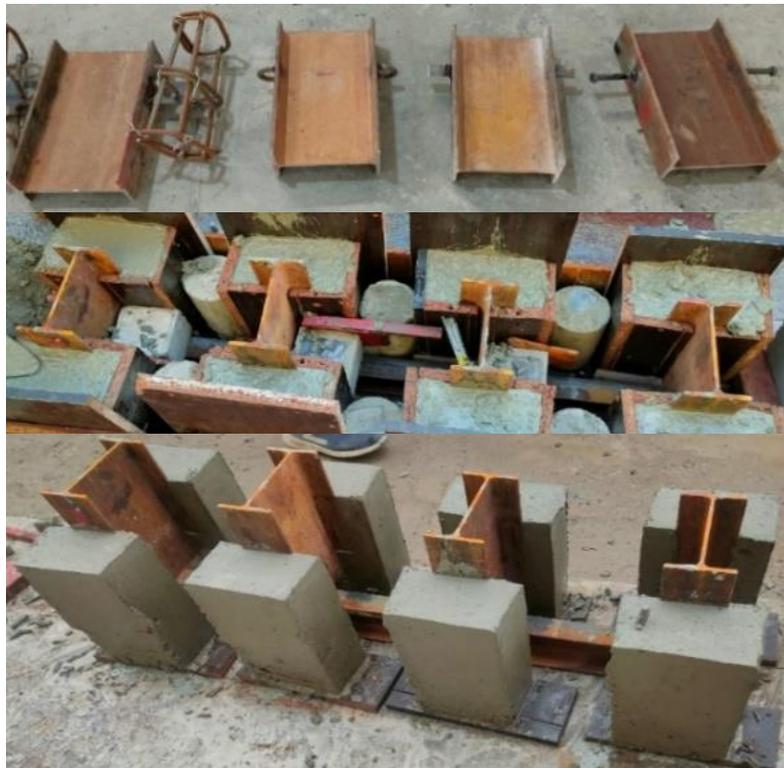
**Fig. 13** Push-Out Sample Casting Process.
