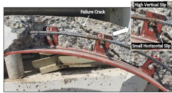
**Fig. 23** High Vertical Slip in Connector C2.
