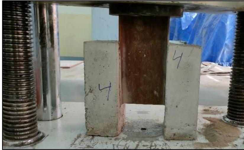
**Fig. 14** Push-Out Test.
