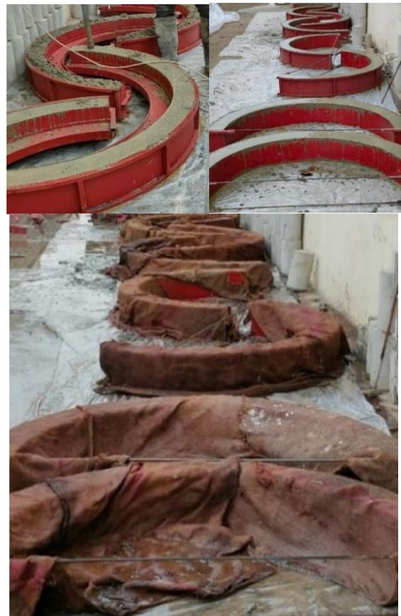
**Fig. 10** Casting and Curing of the Samples.
