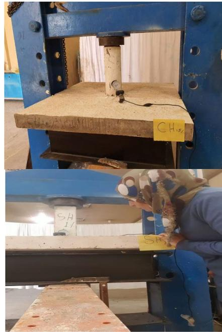
Plate 3 Testing of Slabs.
