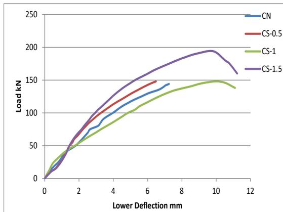
**Fig. 5** Load-Column Deflection Relationship for Slabs of Circular Column Section.
