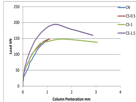
**Fig.3** Load-Column Penetration Relationship for Slabs of Circular Column Section.
