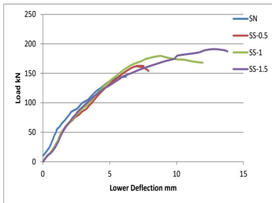
**Fig. 6** Load-Column Deflection Relationship for Slabs of Square Column Section.
