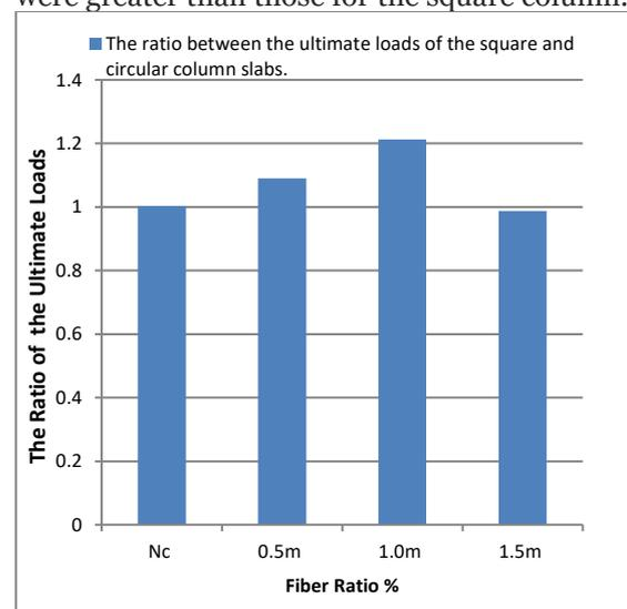
**Fig. 7** Impact of the Ratio Between the Ultimate Loads of the Square and Circular Column Slabs with the Fiber's Ratio.
