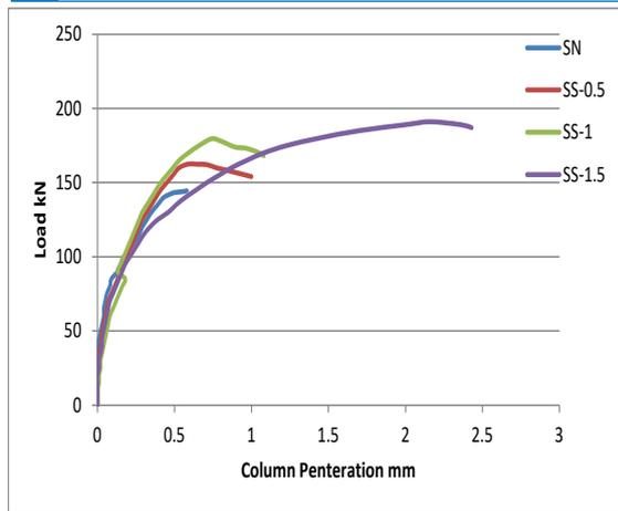
**Fig. 4** Load-Column Penetration Relationship for Slabs of Circular Column Section.
