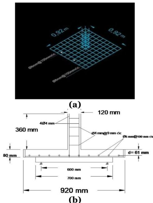
**Fig.1** Details of Specimens Cross-Section (a) Reinforcement Three-Dimension View and (b) Section in a Slab.
