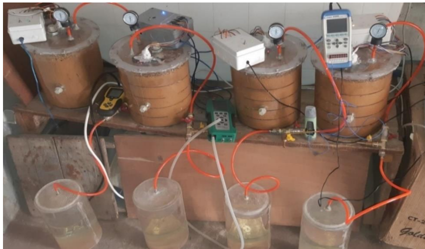
Fig. 5 Photograph of Domestic Anaerobic Digesters Set-up.
