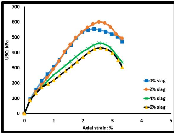
**Fig.3.** Stress vs. strain relationships of iron slag treated soils.
