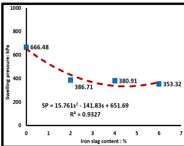
**Fig.6.** Swelling pressure vs. iron slag content
