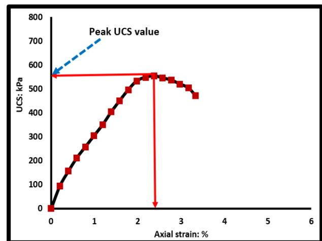
**Fig.2.** Stress vs. strain relationship of untreated expansive soil sample
