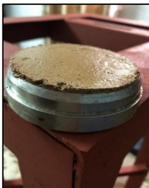
**Fig. 4.** Soil Sample in the Oedometer test
