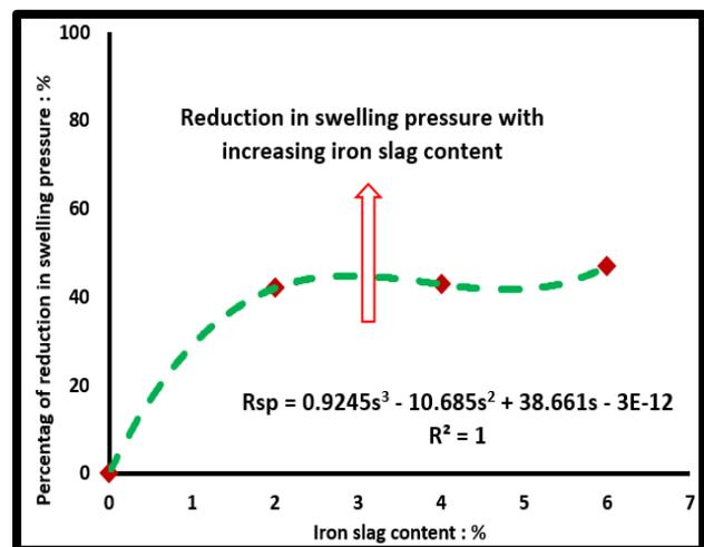
**Fig.7.** Percentage of reduction in swelling pressure vs. iron slag content
