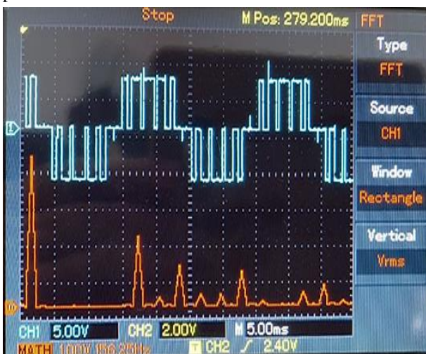
Fig. 15. Output voltage and frequency spectrum for elimination of 3 rd , 5 th , 7 th and 9 th harmonics. (156.25Hz/div)
