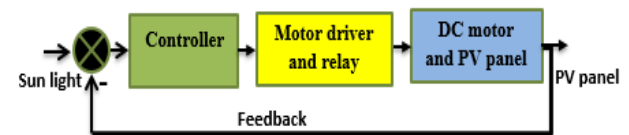
Fig.2. Block diagram of a Dual-Axis Tracking System [12]
