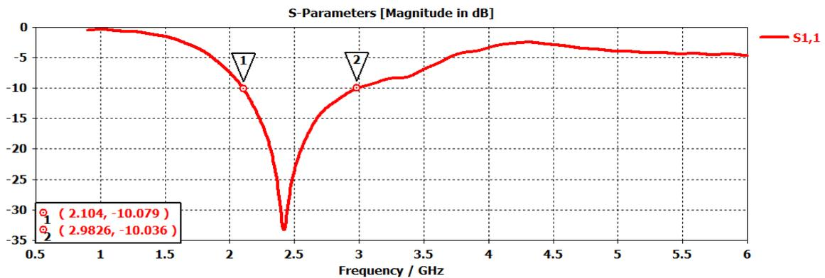
Fig. 3. Return loss versus frequency
