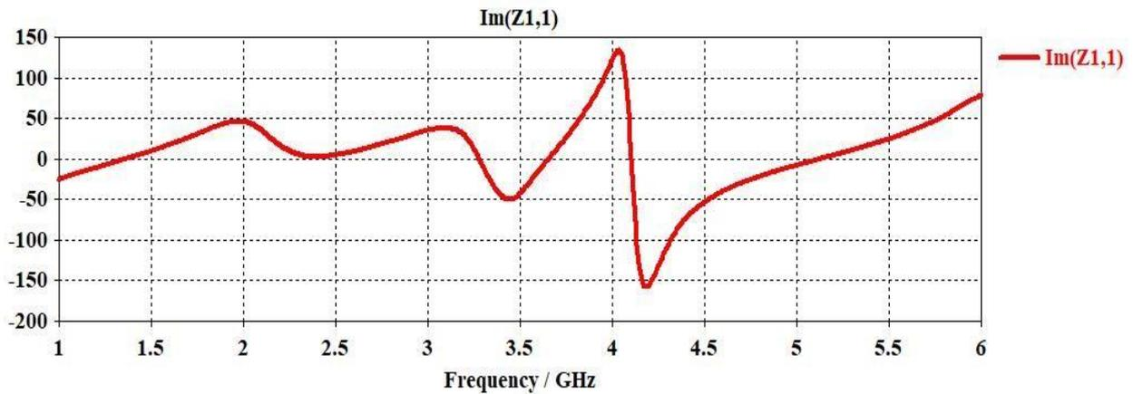
Fig.5. Simulation input resistance (b) imaginary part
