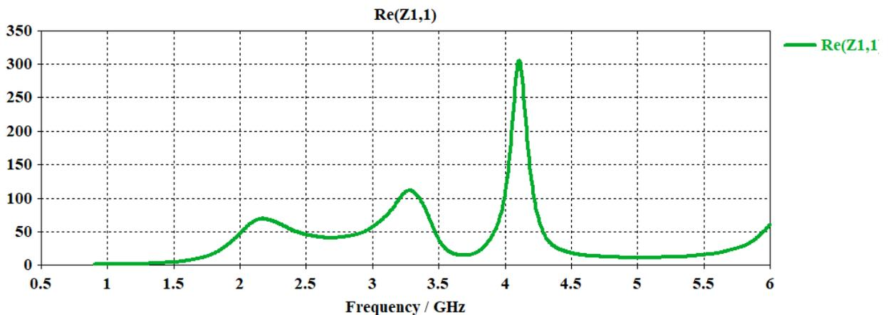
Fig.5. Simulation input resistance (a) real part
