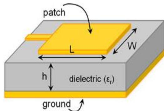
Fig.1. Microstrip antenna configuration
