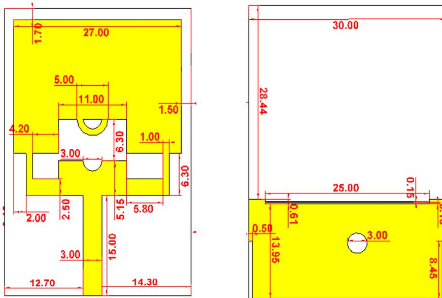
Fig. 2. The geometry of the patch and partial ground antenna
