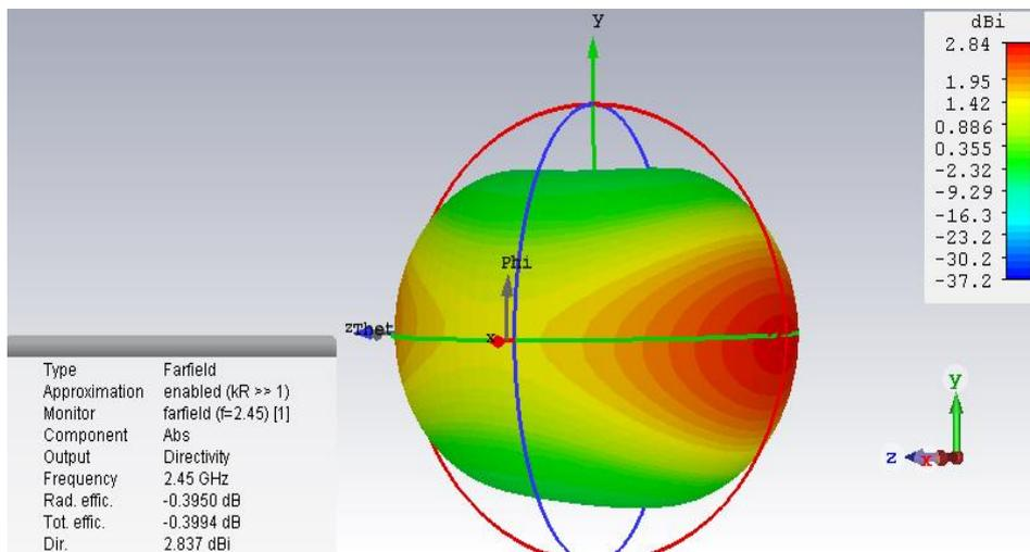
Fig.7. Radiation pattern with total antenna directivity
