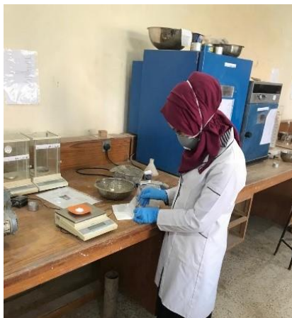
Fig. 4. Prepared soil samples mixed with nanomaterials for direct shear test and double oedometer test.
