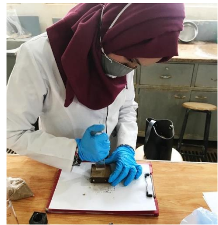
Fig. 4. Prepared soil samples mixed with nanomaterials for direct shear test and double oedometer test.
