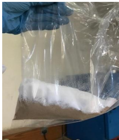
Fig. 4. Prepared soil samples mixed with nanomaterials for direct shear test and double oedometer test.
