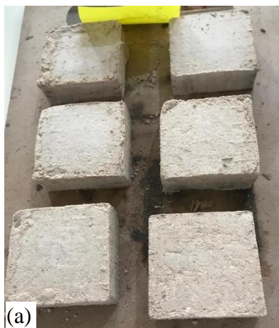
Fig. 3: Prepared gypseous soils for (a) the direct shear test, (b) double oedometer test.
