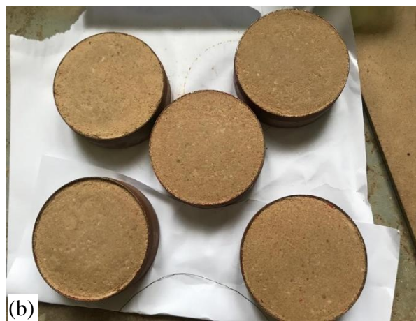
Fig. 3: Prepared gypseous soils for (a) the direct shear test, (b) double oedometer test.
