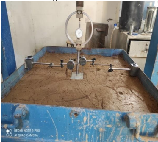
Plate 3. Testing soaked gypseous soil.
