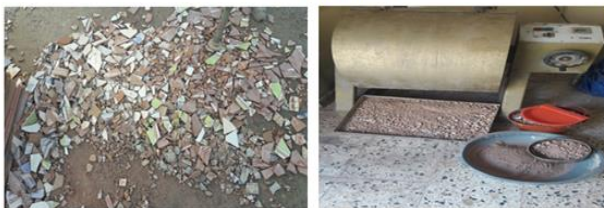
ceramic crushing and grinding stages
