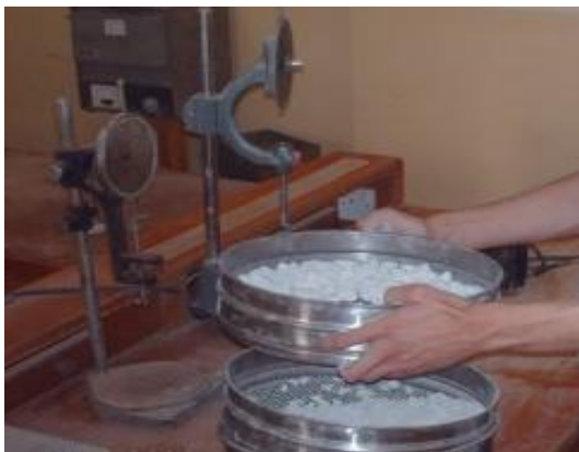
Fig. (3) : Sieve analysis test
