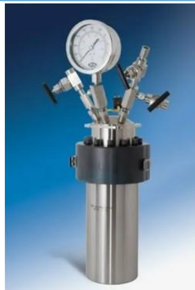
Fig. 1 The Parr 4682 Type High-Pressure Homogeneous Chemical Reactor.
