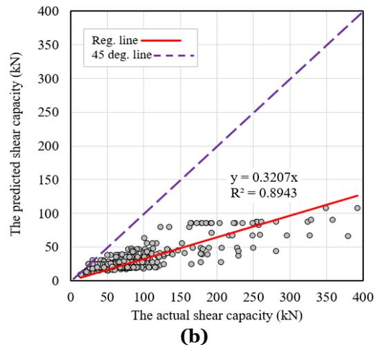
**Fig. 4** Comparison between Measured and Predicted Shear Capacity of RC Beam without Web Reinforcement Using Linear Regression Model (LR). (a) Full Model and (b) Simplified Model.
