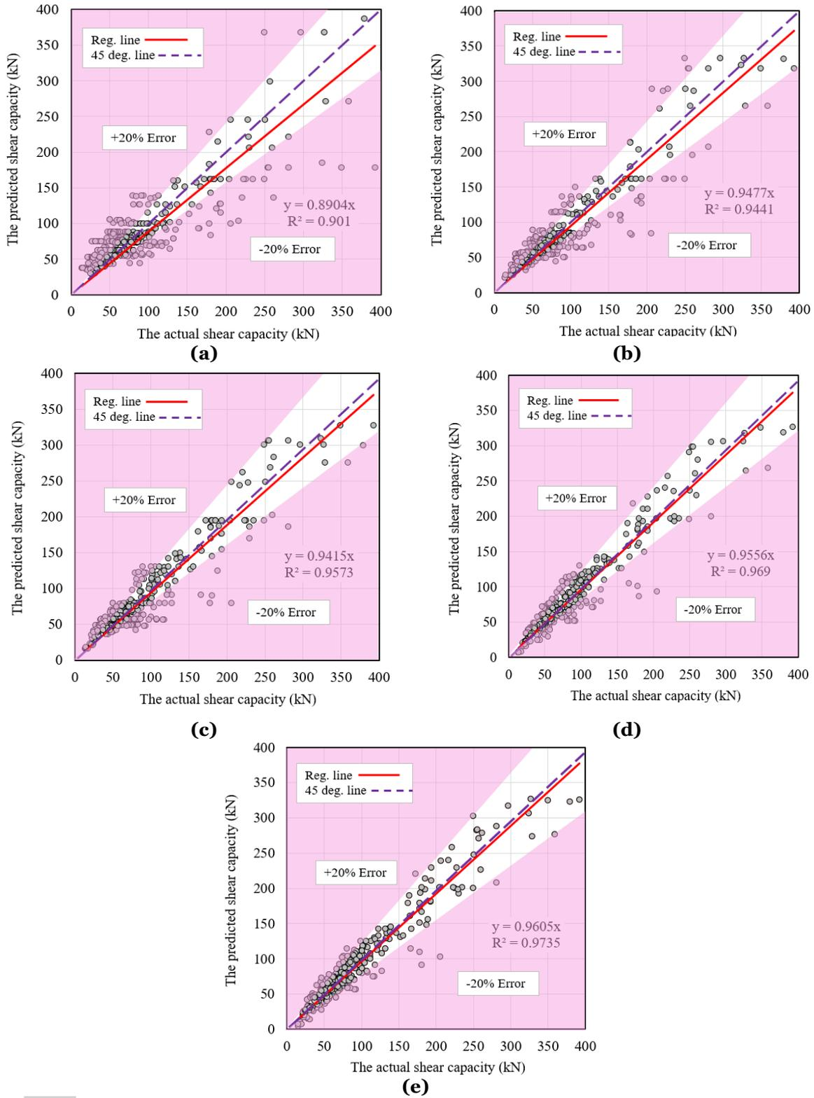
**Fig. 5** Comparison between Measured and Predicted Shear Capacity of RC Beam Without Web Reinforcement Using Stepwise Multivariate Regression (SMR) (a) Model 1, (b) Model 2, (c) Model 3, (d) Model 4, and (e) Model 5.
