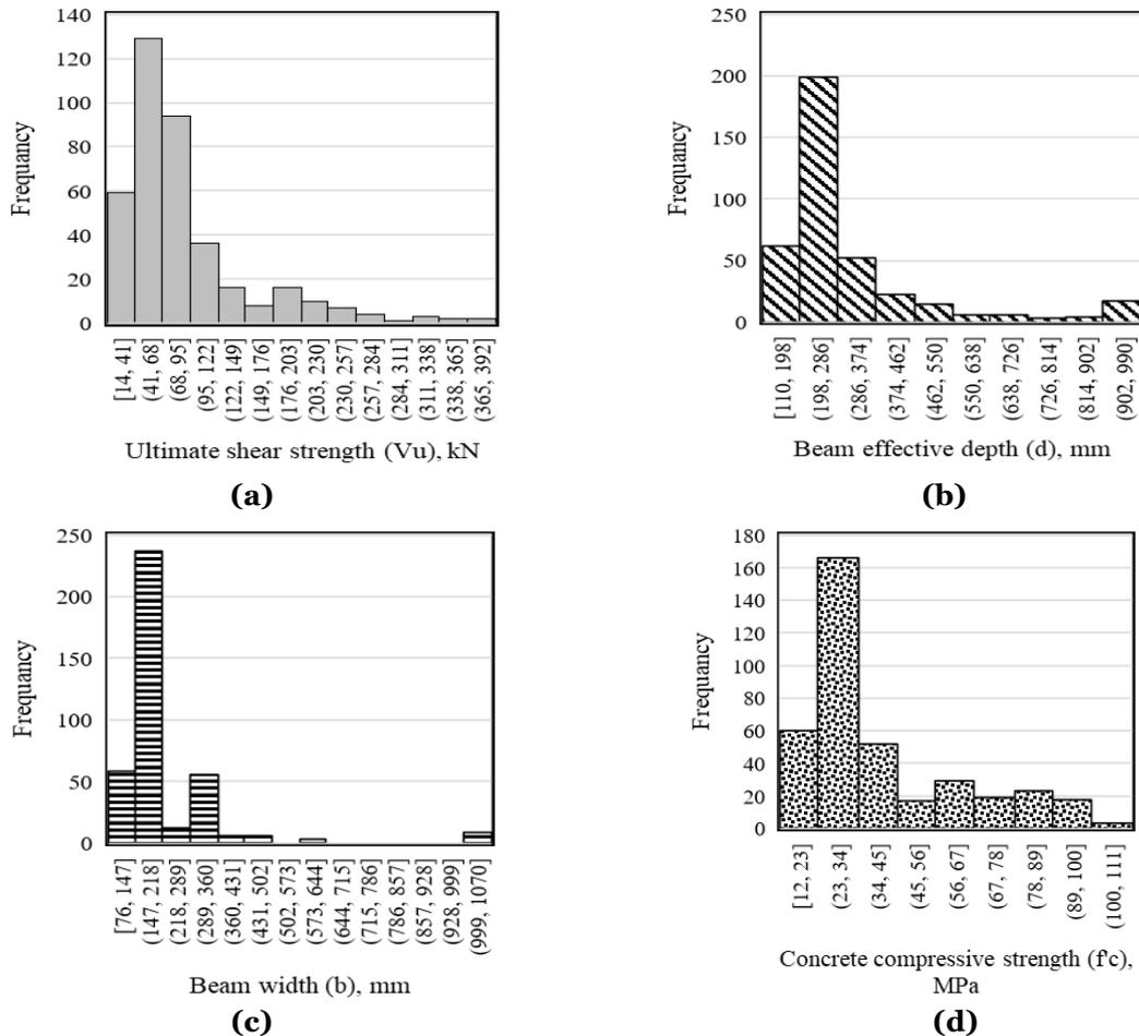
**Fig. 1** Frequency Distribution of (a) the Shear Capacity ( $V_u$ ), (b) Effective Beam Depth, (c) Beam Width, and (d) Concrete Compressive Strength of the Beams Used in this Study Beam.
