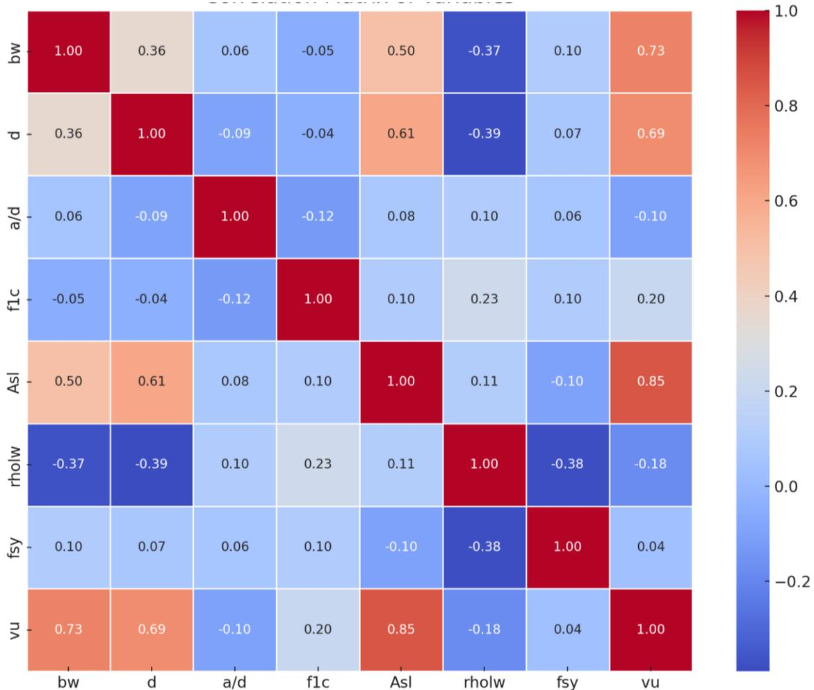
Fig. 2 Correlation Matrix of Structural Parameters Affecting Shear Capacity (Vu).
