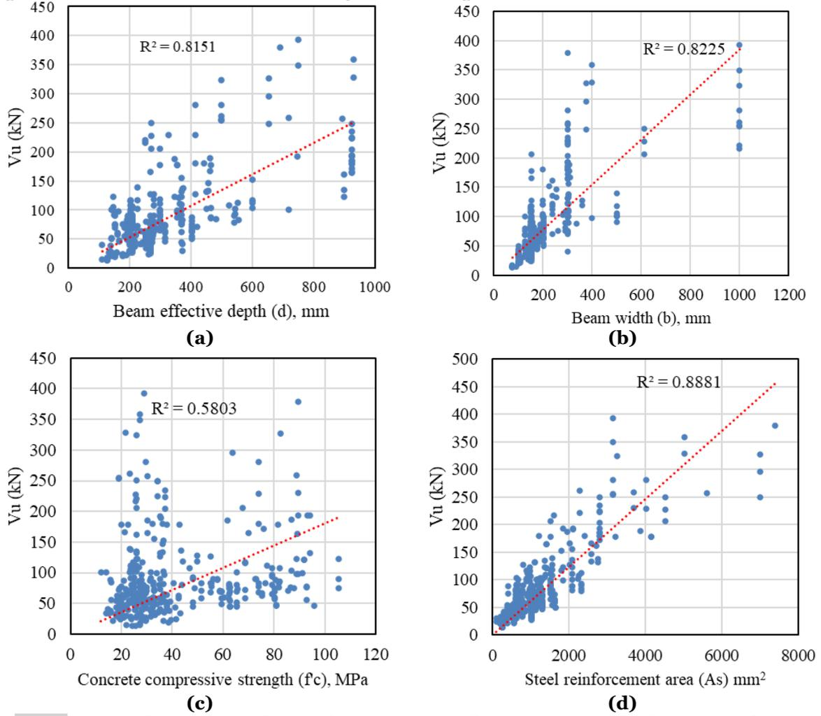
**Fig. 3** Scatter Plots and Correlation of  $V_u$  Versus (a) Effective Beam Depth, (b) Beam Width, (c) Concrete Compressive Strength, and (d) Steel Reinforcement Area.
