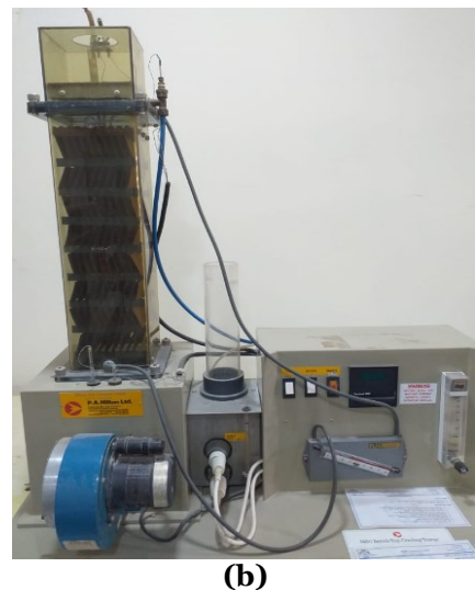
Fig. 1 Test Rig (A) Illustrative Diagram (P. A. Hilton Cooling Tower Model H891). (B) Lab Apparatus.
