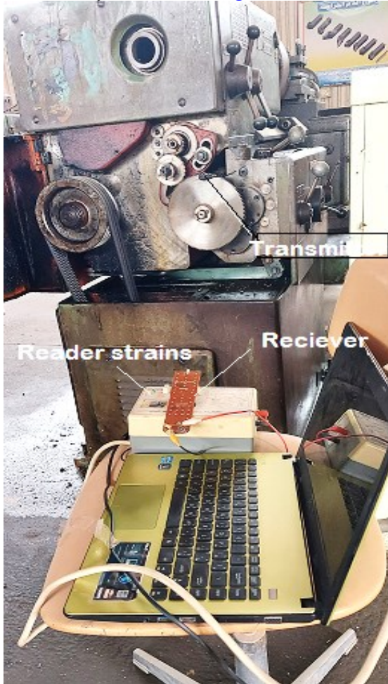
Fig. 11 Experimental Apparatus to Measure Strain.
