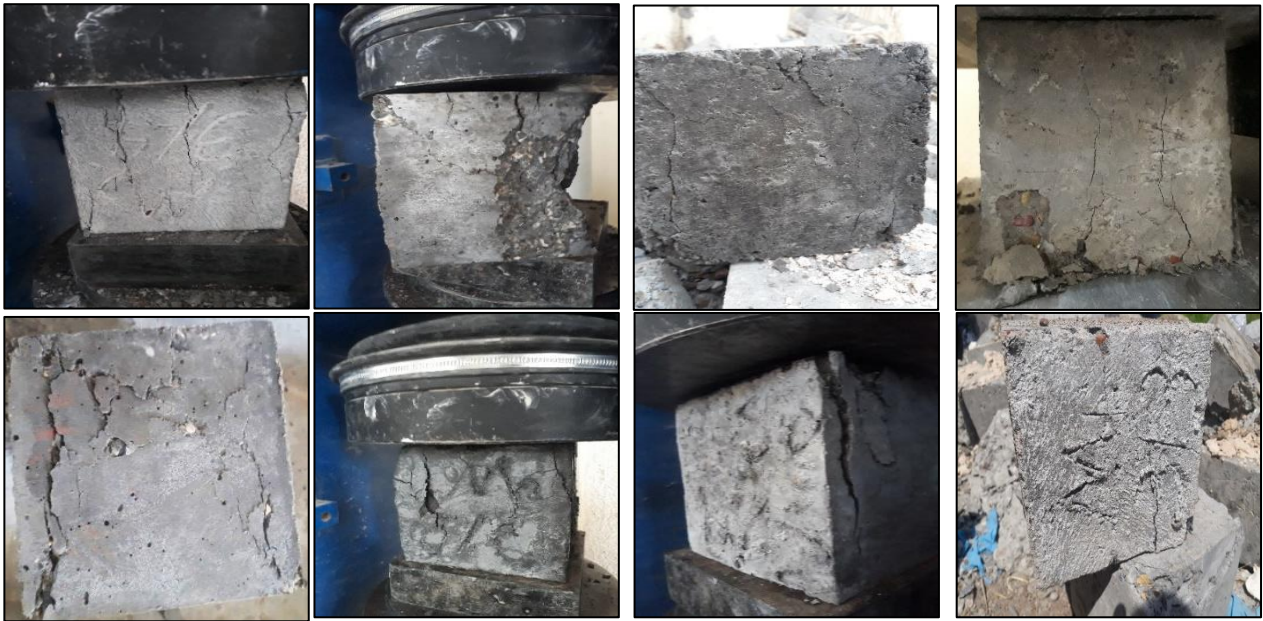
Plate.5. Compressive Strength Failure
